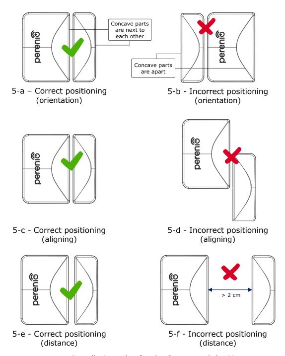
Figure 5 – Installation rules for the Sensor and the Magnet
