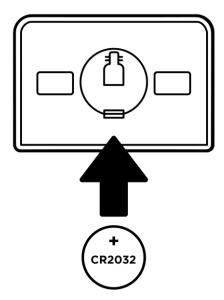
Figure 7 – Positioning of the battery in the Door & Window Sensor
