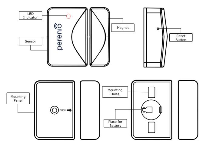
Figure 2 - Door & Window Sensor Components
