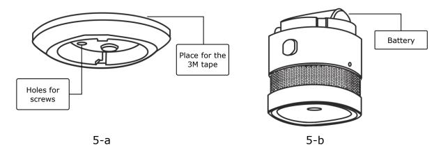
Figure 5 – Fastening of the Smoke Sensor on screws or the 3M tape
