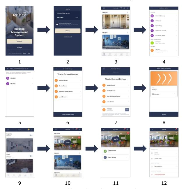
Figure 7 - Add new device (Sensor) procedure
