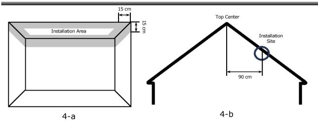
Figure 4 - Installation of the Smoke Sensor on a flat and sloping ceiling
